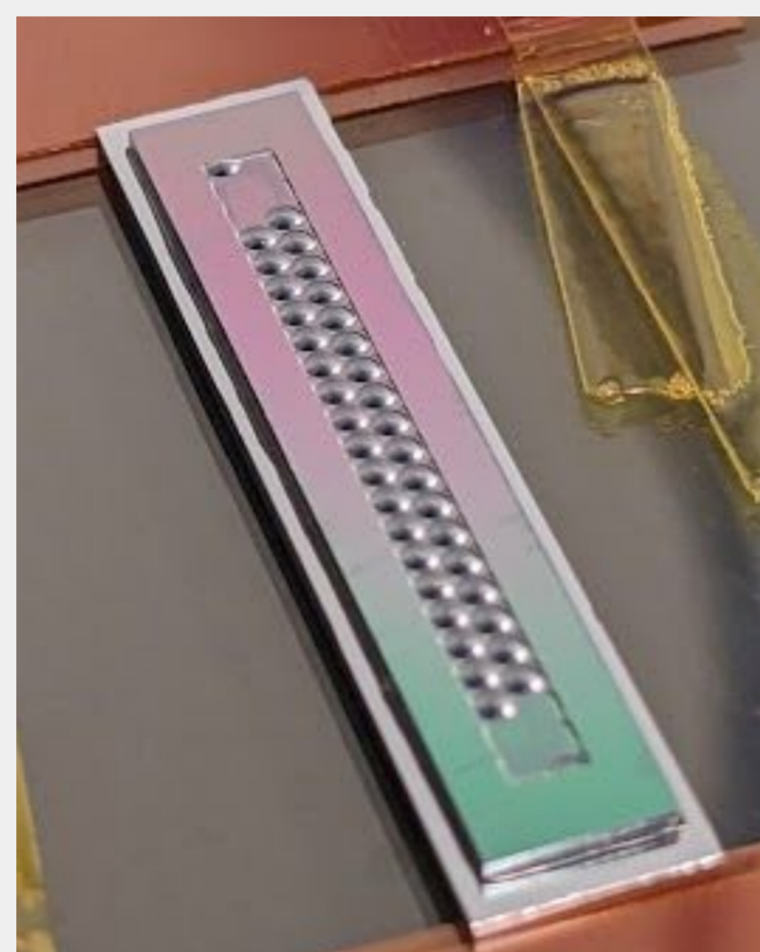
Above: Photograph of \lambda \sim 25 \mu\text{m} hybridized microlens array. Below: FLIR photographs showing prototype hybridized arrays with (right) and without (left) inclusions.
