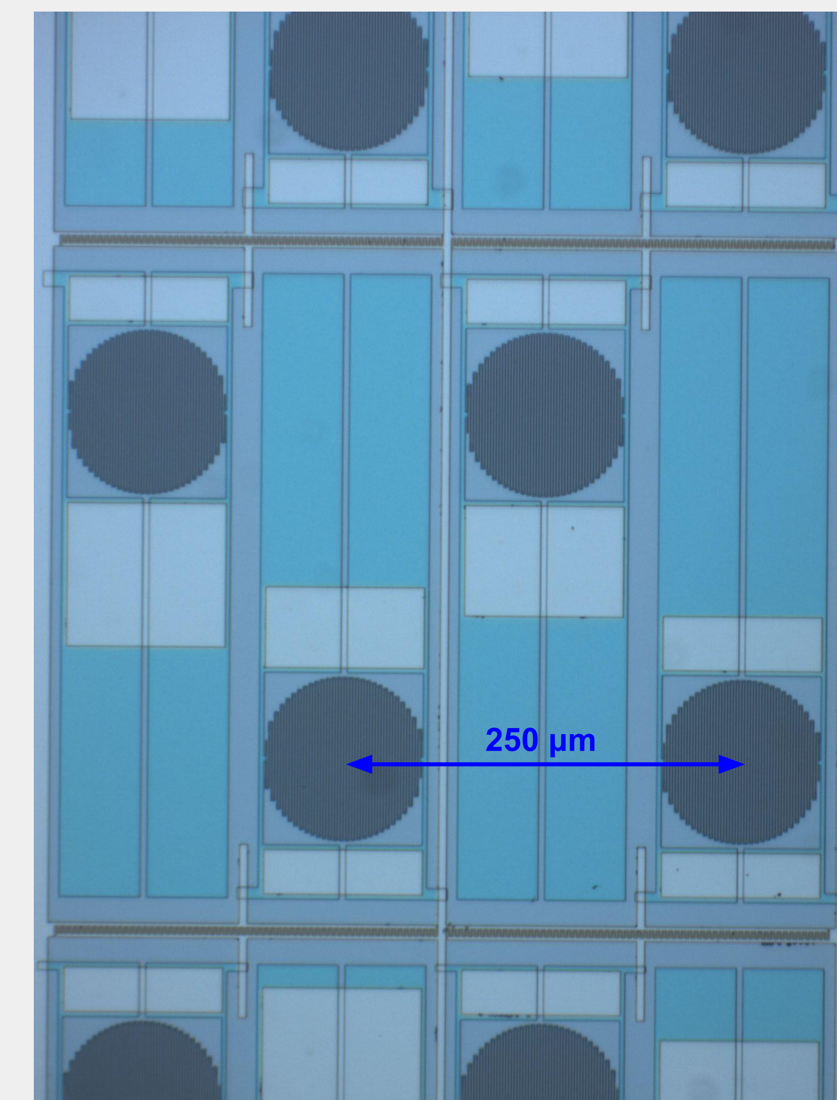
PPC KIDs. A meandered TiN inductor comprises the absorber. Unique capacitors define the unique resonant frequency of each detector.
