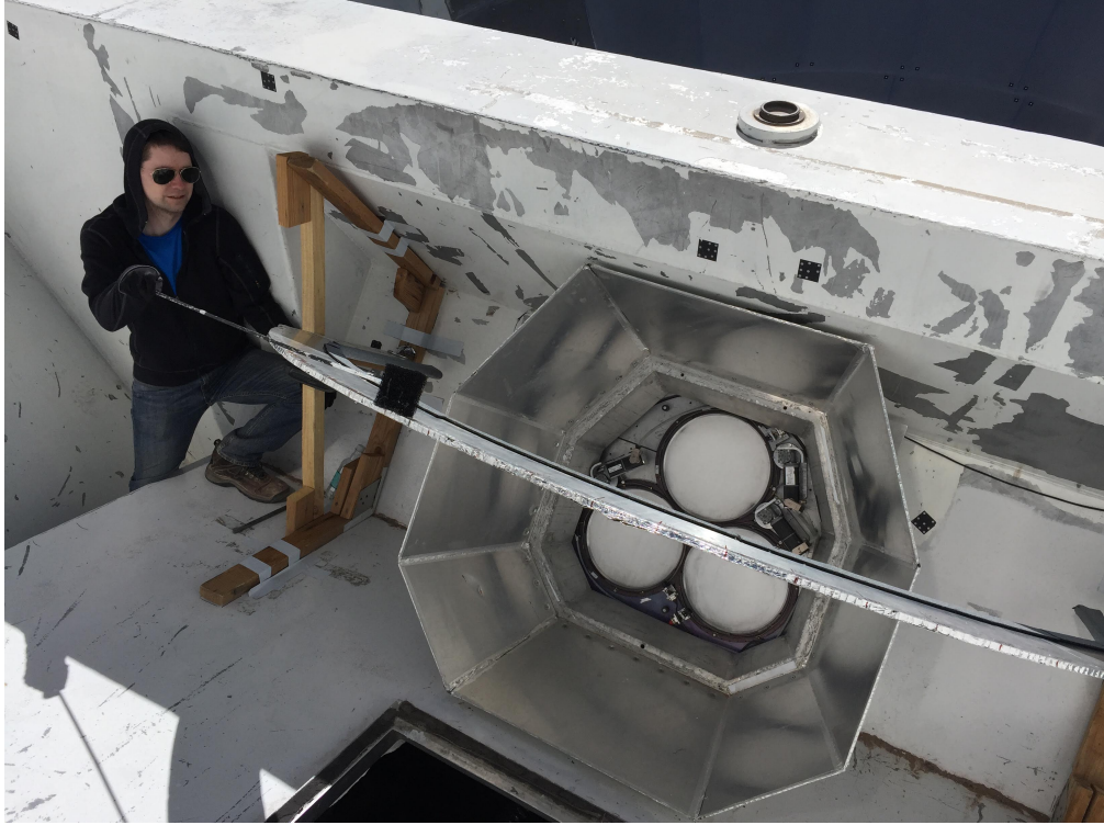
Figure 2.4: Photograph of the author performing Eccosorb-Stick beam mapping measurements of AdvACT’s MF2 array (the top receiver window). The author stands far to the side of the beam, against the bulkhead wall and moved the Eccosorb HR-25 block into and out of the the beam. A hexcell arch with every 5° marked from -60^\circ to +60^\circ is used as a ruler/guide for Eccosorb placement. The arch is centered and leveled with the MF2 optical axis. Note the hexcell receiver baffle installed around the windows to prevent warm spillover at wide angles.
