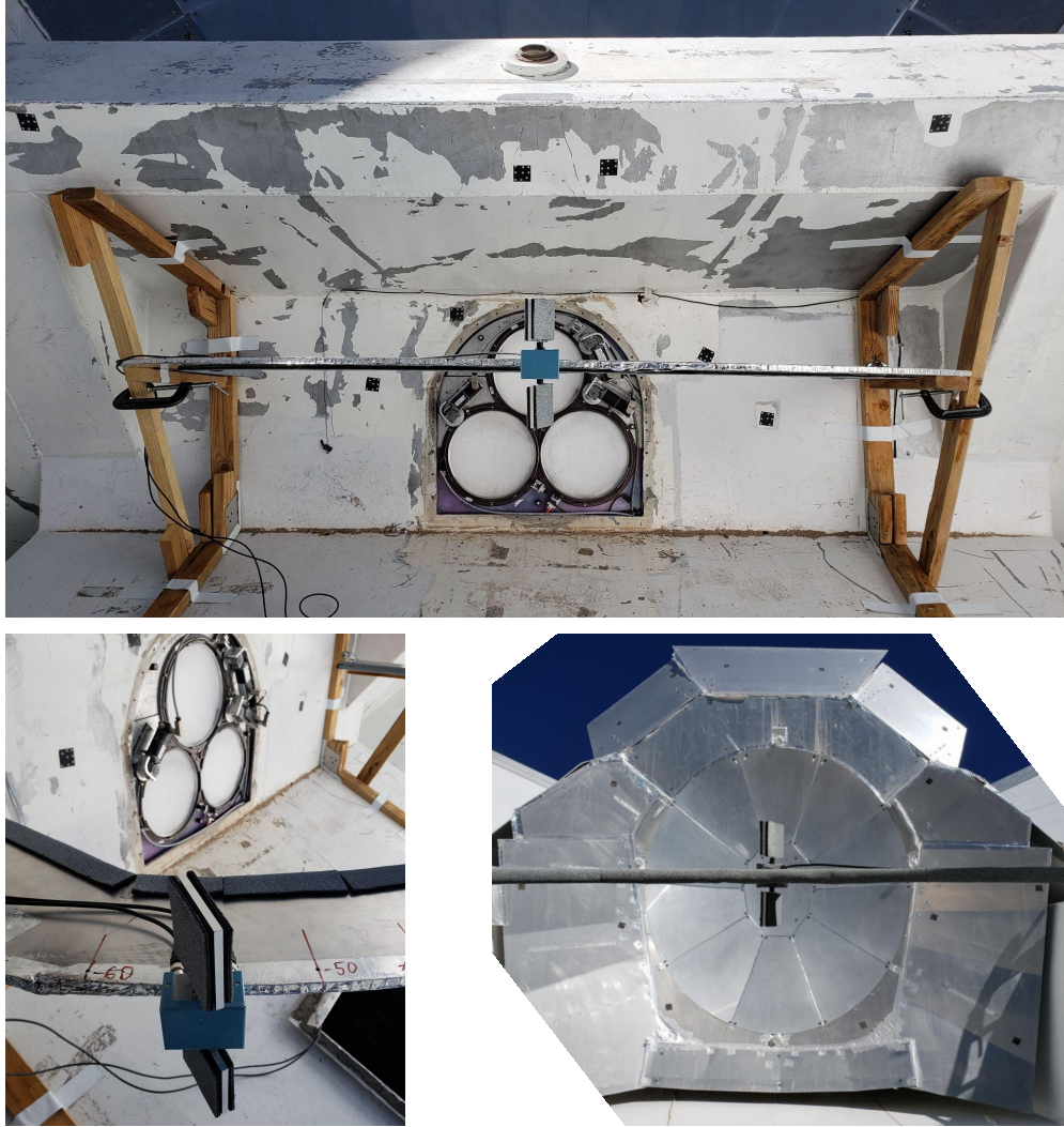
Figure 2.5: Photographs of the Eccosorb-Robot method. Two Eccosorb AN-72 paddles were rotated by a stepper motor at each of the 5^\circ increments on the same hexcell arch used in the Eccosorb-Stick method. The upper panel shows the arch and robot directly in front of the MF2 window. The bottom left panel shows the robot mounted at -55^\circ from MF2's central optical axis. The lower right panel shows the view of the arch, robot, and secondary mirror from the perspective of MF2. The 3" square paddles horizontally span \sim 3^\circ of the receiver beam.
